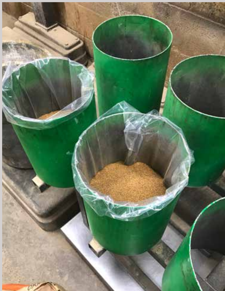
Plastic bag-lined cylinders isolate ingredients until they are poured into finished feed.
