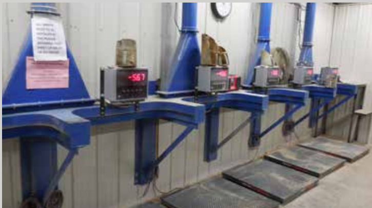
A camera is pointed towards these scales and large digital readouts, creating a visual record of medications and amounts for each feed order.
